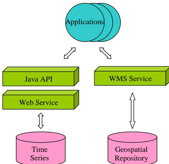
Figure 7 Schematic design of the data storage used for hydrological data
