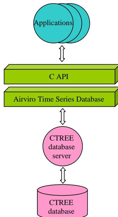
Figure 4 Schematic design of the Airviro time-series database (C API stands for Application Programming Interface written in C)
