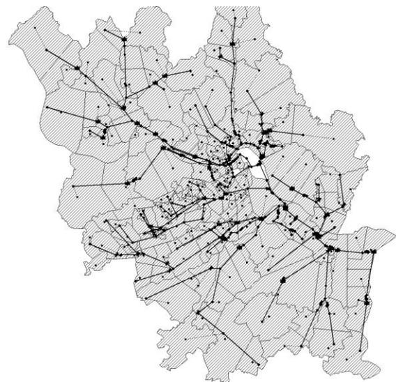
**Figure 2: Overview of the aggregated Linz catchment model in SWMM 5**
